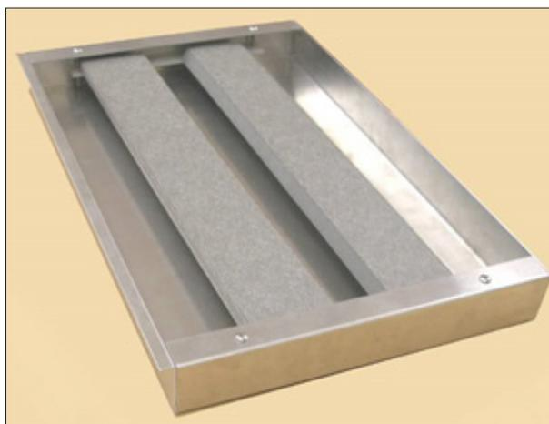
Figure 12.3l: Wide specimen holder with clamps.
