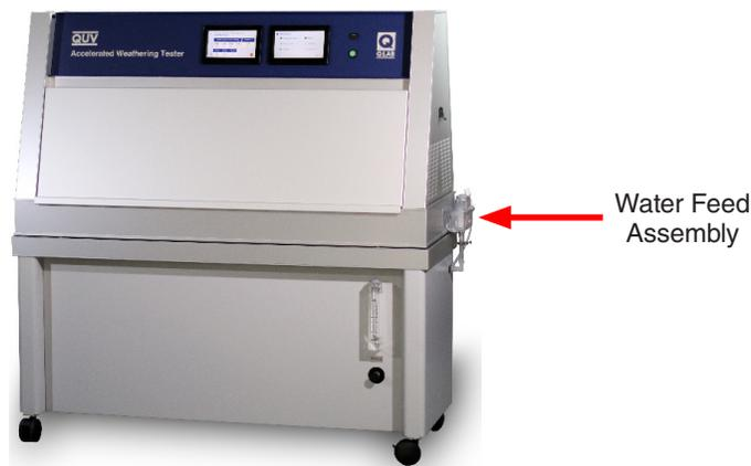
Figure 6.4a: QUV water supply connection location.
