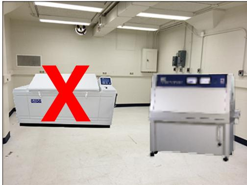
Figure 4.2a: Do not install QUV testers in a room with corrosion chambers.
