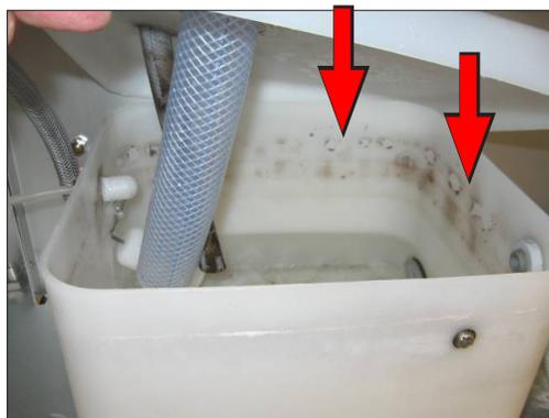
Figure 16.5g: Reservoir lid removed showing mold growth.
