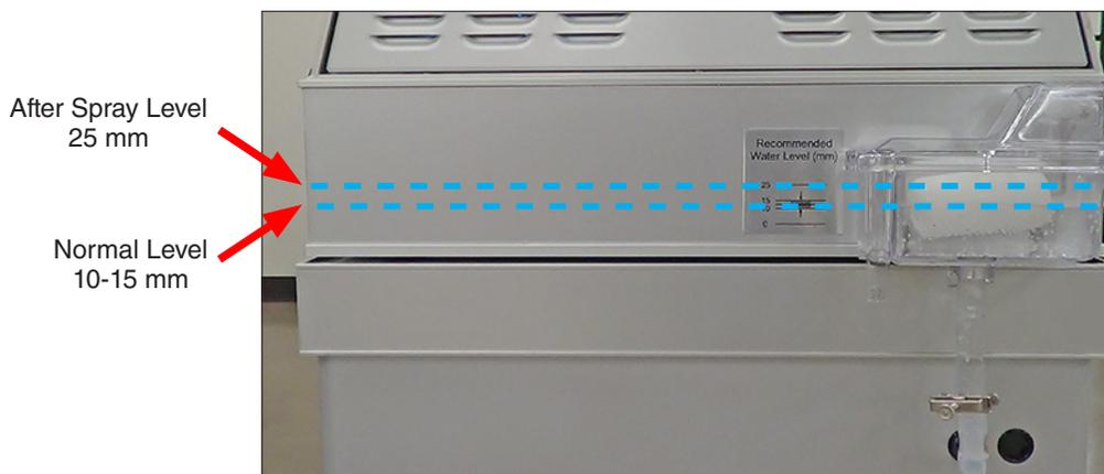
Figure 6.4h: Normal and after spray water levels.
