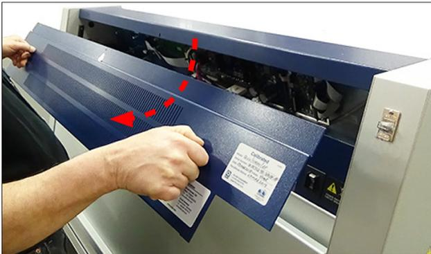
Figure 11.1a: Remove the QUV rear access panel from the control top to access the main controller and electronics.
