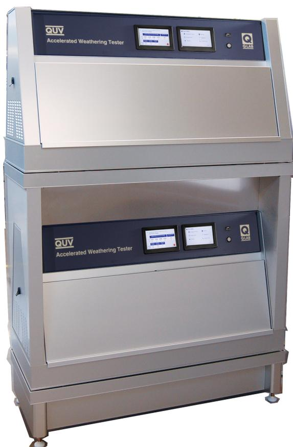
Figure 15.1a: QUV testers without spray on space saver frame.
