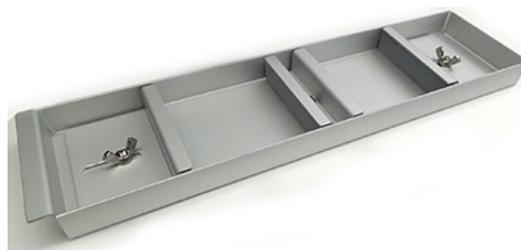
Figure 12.3k: Narrow 3D specimen holder with clamps.
