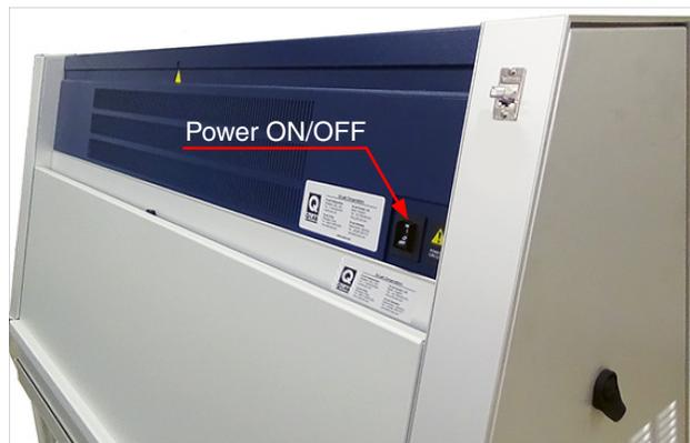
Figure 11.2a: Power switch location.
