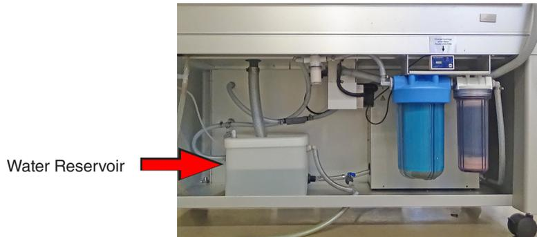
Figure 16.5e: Integrated water repurification system.
