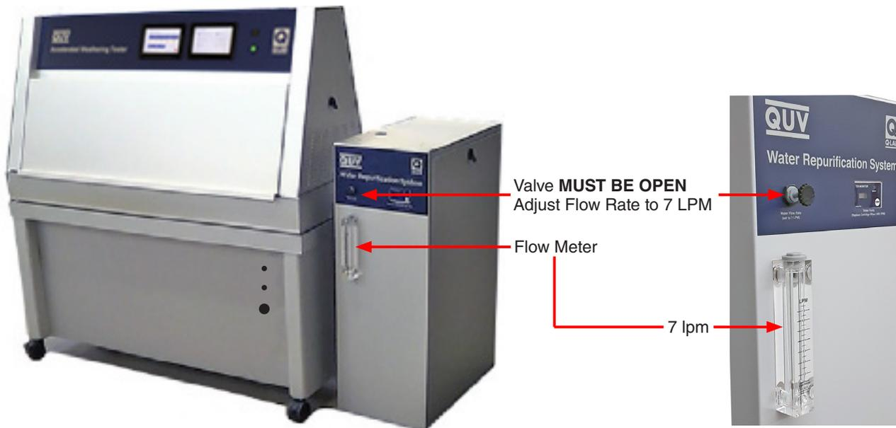
Figure 15.3d: QUV spray tester with standalone water repurification system (V-60160-K).
