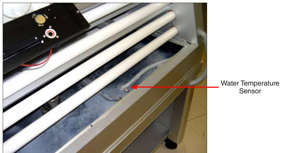
Figure 10.3: Water temperature sensor location (shown with specimens and water pan cover removed).
