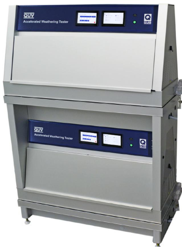
Figure 15.1b: QUV testers with spray on space saver frame.
