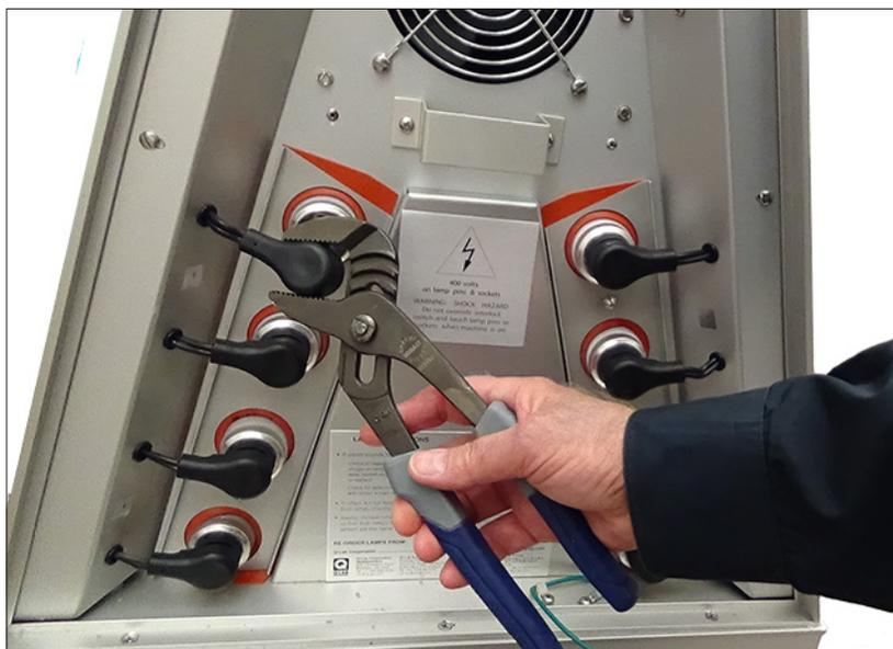
Figure 17.4: Squeeze gently to tighten socket.
