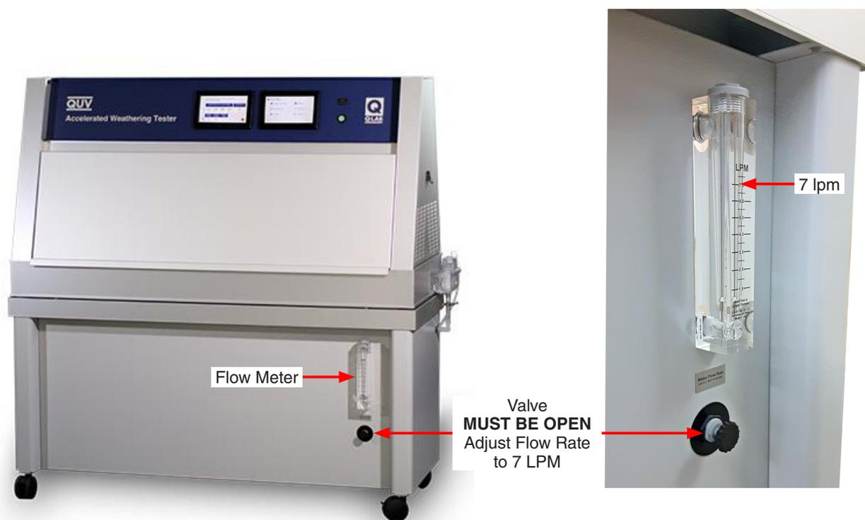
Figure 15.3b: Integrated water repurification system flow adjustment valve and flow meter.
