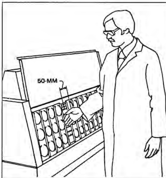
Figure 1B. One sample holder removed. Hand 50 mm from lights (same as sample): allowable daily exposure is 1 minute for UV-B lamp.
