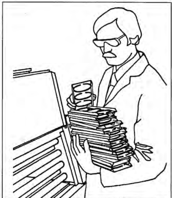
Figure 38. All 26 panel holders stack conveniently for carrying to another room for sample analysis. Simply cradle them in your arm and stack, alternating flanges up and flanges down.
