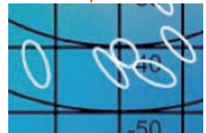
The major axis of the white ellipse representing the color discrimination threshold of the human eye is not in the direction of saturation.
