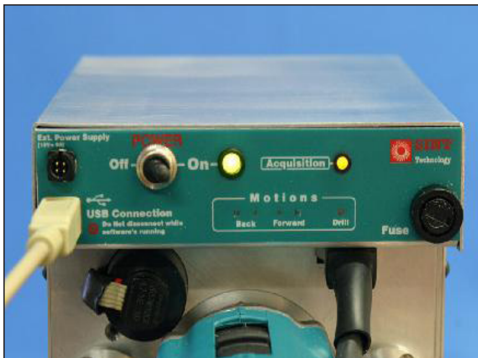
Figure 2.3: USB lead connecting to PC (left) with correct displays lighting up. Machine is ready to use (SINT 2007)
