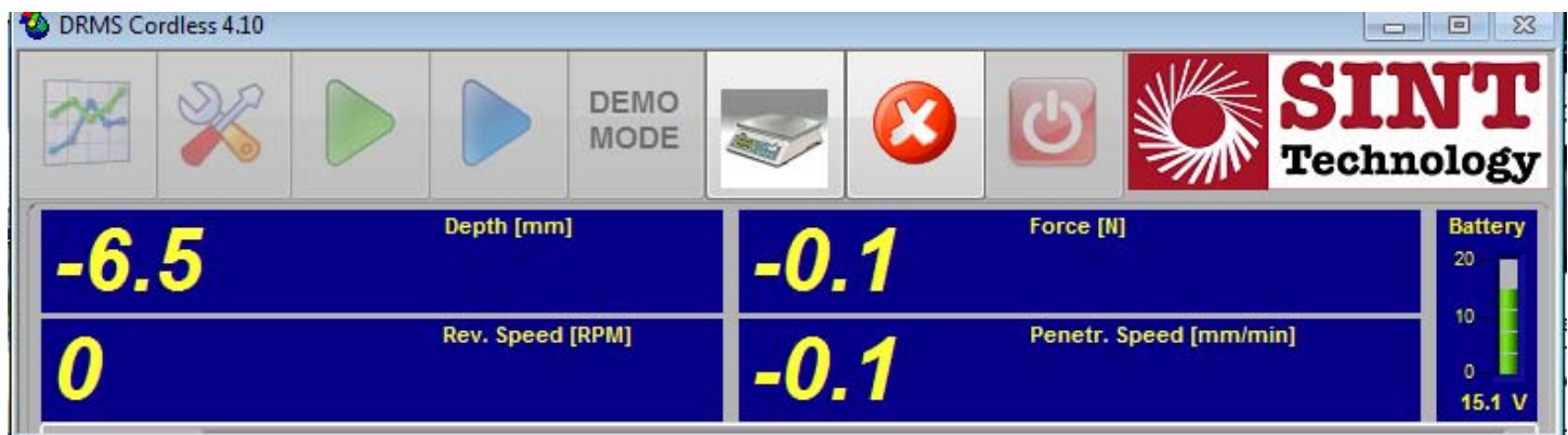
Figure 3.5: Signal Monitor. NOTE: Moving the drill by pulling the trigger will adjust the depth accordingly (SINT 2007)
