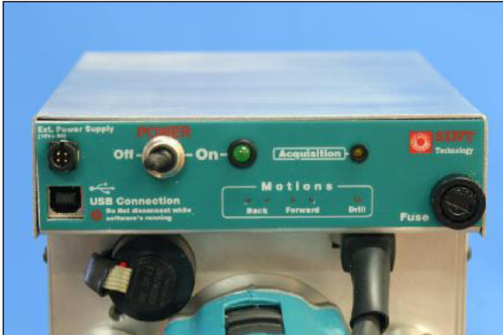
Figure 2.2: Main panel on the mechanical instrument including yellow “Acquisition” light and green “ON” light (SINT 2007)
