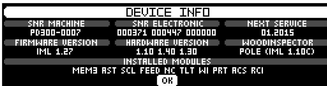
Details of your instrument can be displayed by selecting the device information symbol in the main menu. The serial number of the instrument as well as the serial numbers of the electronic unit are shown in this menu. Furthermore the next service date, the versions of the firmware, of the hardware and of the WoodInspector are listed. The installed Add-on modules are also displayed in the device information menu.
