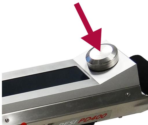
Press the navigation knob to switch on the instrument and keep it pressed until the IML logo appears in the display.
