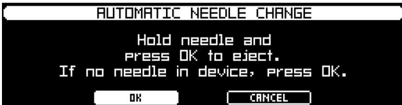
Hold the blade of the drilling needle with the universal pliers and press the **OK** button. If no needle is in the machine, press also the **OK** button.
