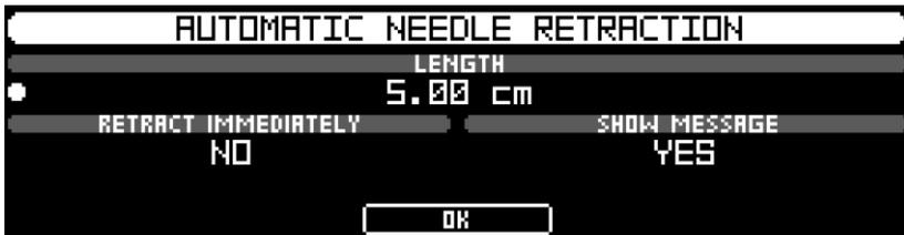
The option **LENGTH** determines which minimal length the cavity must have to activate the automatic needle retraction.
