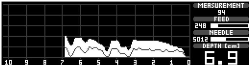
On the left side is shown the preview curve. As shown in the picture above, the drilling curve (bright and filled) is displayed simultaneously with the feed curve (dark and not filled). The drilling curve is always displayed brightly and the feed curve (additional module) a little bit darker.
