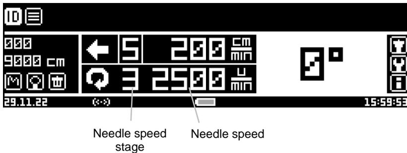
The advanced mode additionally shows the rotational needle speed.
