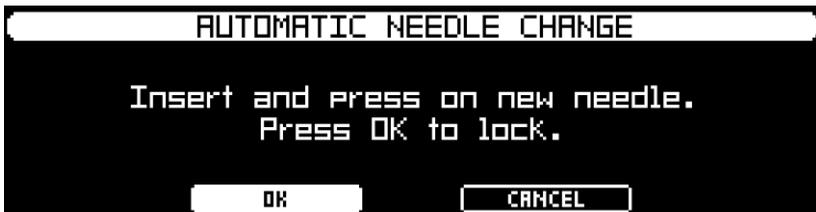
Remove the old needle of the instrument and insert a new one. Hold the new drilling needle on the blade with the universal pliers (like you did when you removed the needle) and press on the needle against the chuck. Now press the button **OK**.
