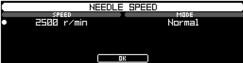
In normal mode you can choose a rotational speed for the drilling needle between 1500 rpm and 5000 rpm.
