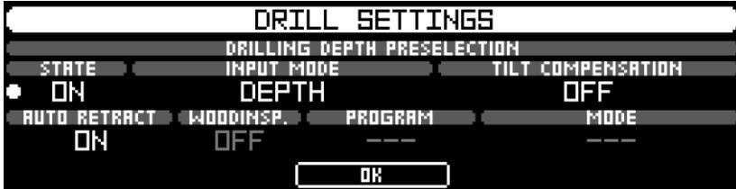
Use the **DRILLING DEPTH PRESELECTION** feature to set the drilling depth individually. (See chapter 4.6.1) Once the preselected depth is reached the drilling needle retracts automatically.
