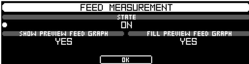
With **STATE** you can opt for recording the feed force while measuring or not. If you have activated this option the free recording length reduces by half.
