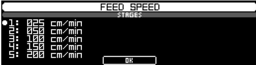
Each of the 5 feed speed stages is pre-adjusted. The picture above shows the standard adjustment.
