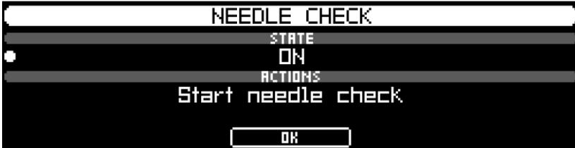
**STATE** indicates if the needle check is on or off. If needle check is enabled, the needle will be checked before every drilling and the needle state will be shown. The result (good or bad) will be saved together with the measurement and will be displayed in PD-Tools after the transmission to the computer.
