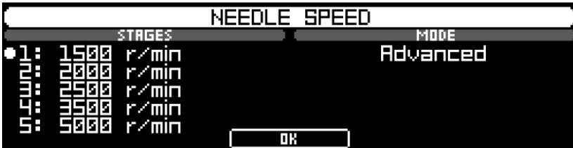
Each of the 5 rotational speed stages is pre-adjusted. The picture above shows the standard adjustment.
