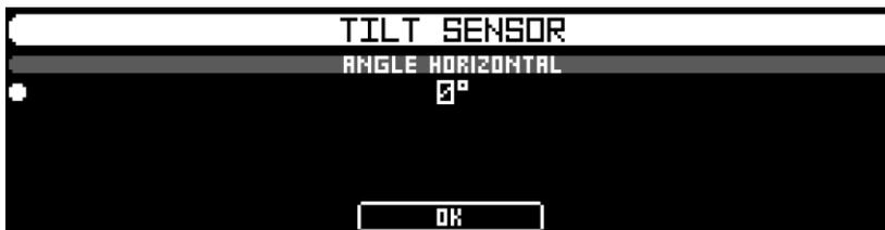
The option **ANGLE HORIZONTAL** determines if the angle  $0^\circ$  or  $90^\circ$  is displayed when the device is aligned horizontally. Select **0°** and the display will be in the range between  $-90^\circ$  (unit tilted forward) and  $+90^\circ$  (unit tilted backwards). Select **90°** and the display will be in the range between  $0^\circ$  (unit tilted forward) and  $180^\circ$  (unit tilted backwards).
