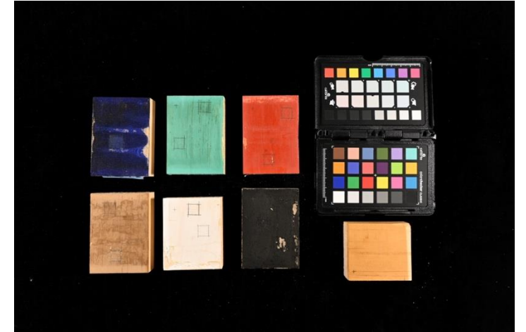
▲ Modified Method Samples Before Accelerated Weathering Test
