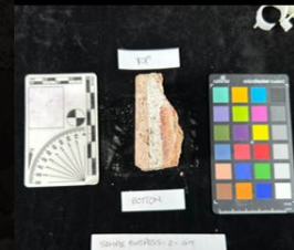
Figure 24: 3 samples extracted: Magazine buttress (2) and bastion wall (1). Figure by author, 2025.
