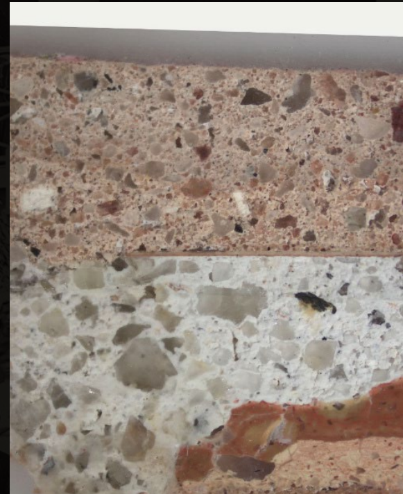
Figure 25: Cross sections of samples extracted showing a mono and multilayer render distribution. Figure by author, 2025.
